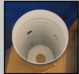
MS7001EA Combustion Liner
